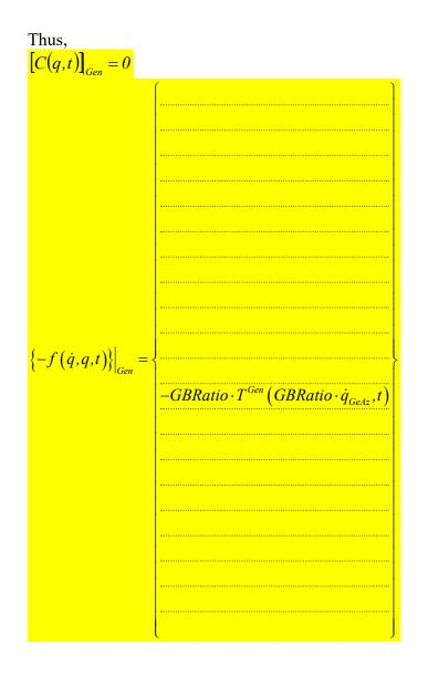
Similarly, the mechanical torque applied to the high-speed shaft from the high-speed shaft brake is applied equally and oppositely to the structure that furls with the rotor. Thus,
