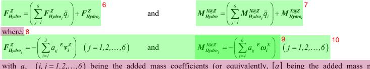
with  $a_{ij}$  (i, j = 1, 2, ..., 6) being the added mass coefficients (or equivalently, [a] being the added mass matrix),  $F_{Hydro_j}^Z$  (j = 1, 2, ..., 6) and <sup>11</sup>  $M_{Hydro_j}^{X@Z}$  (j = 1, 2, ..., 6) being the partial hydrodynamic added mass forces and moments, and  $F_{Hydro_t}^Z$  and  $M_{Hydro_t}^{X@Z}$  being the contributions to  $F_{Hydro}^Z$  and  $M_{Hydro_t}^{X@Z}$  that don't depend on platform accelerations.
